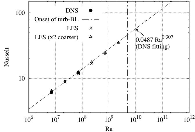
Figure 3:  $Nu$ -vs- $Ra$  results obtained with LES at  $Pr = 0.005$  using the same RBC configuration as in Ref.[8] where the two DNS results (solid black dots) were computed. The vertical dash-dotted line corresponds to the estimated  $Ra$  (for this particular  $Pr$ ) where the thermal boundary layer becomes turbulent.
