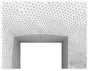
DNS<sup>3</sup> of the turbulent flow around a square cylinder at Re = 22000
