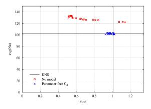
The overall Nusselt number and the centerline stratification for 50 randomly generated coarse grids with fixed stretching at  $Ra = 10^{10}$ .
