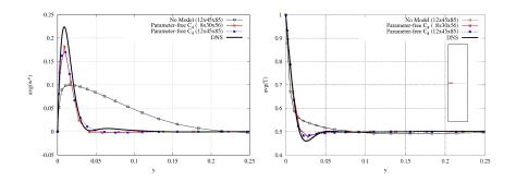
Averaged vertical velocity and temperature profiles at the horizontal mid-height plane.
