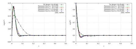
Averaged vertical velocity and temperature profiles at the horizontal mid-height plane at  $Ra = 10^{10}$ .
