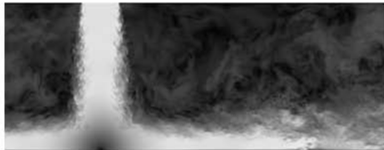
Impinging jet Re=20000 (mesh 100M nodes)
