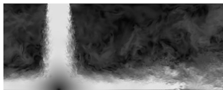
Plane impingement jet at Re = 20000 (102M grid points)
