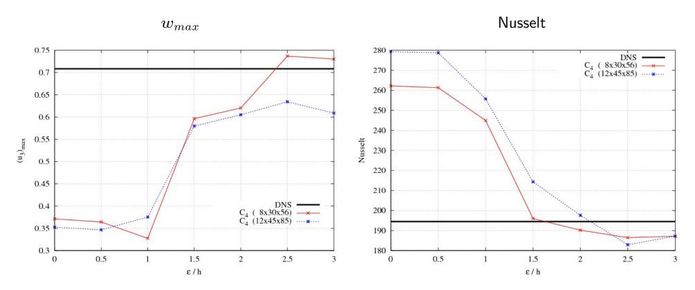
The maximum of the averaged vertical velocity at the horizontal mid-height plane and the overall averaged Nusselt number as a function of the ratio of the filter length  $\epsilon$  to the average grid width h.
